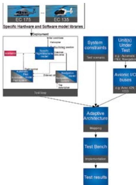
hardware computing resource (FPGA) to build up adaptive avionic test systems. The proposed hybrid architecture for the next avionic test systems is composed of multicore CPUs and FPGAs. Our expectation of the above described architecture is to prototype models that can be eligible and relocated in the FPGA.
