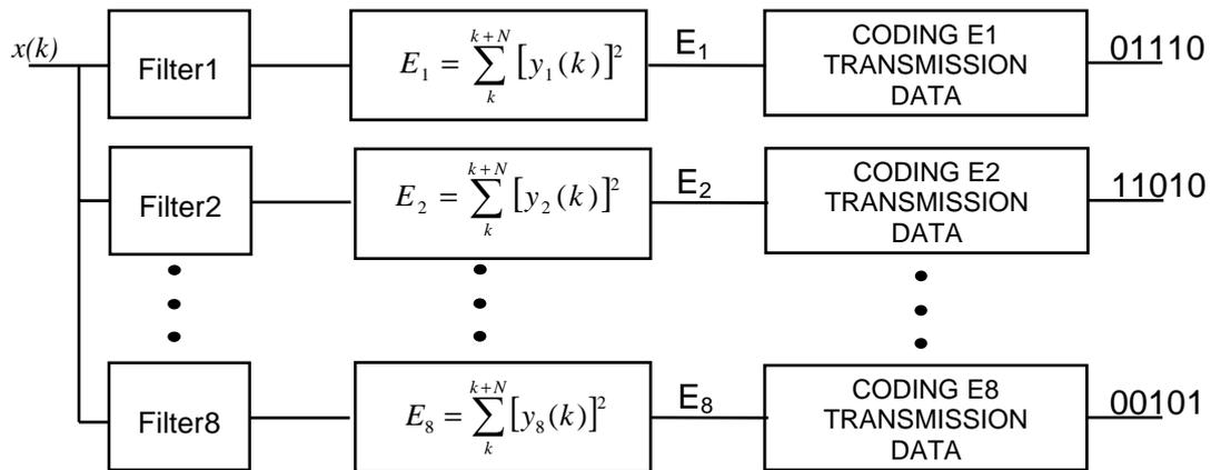
Fig. 5: Filtering, energy calculation and data transmission
